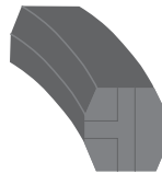
SBX style octagonal, with pressure equalization hole, as per API 17D
